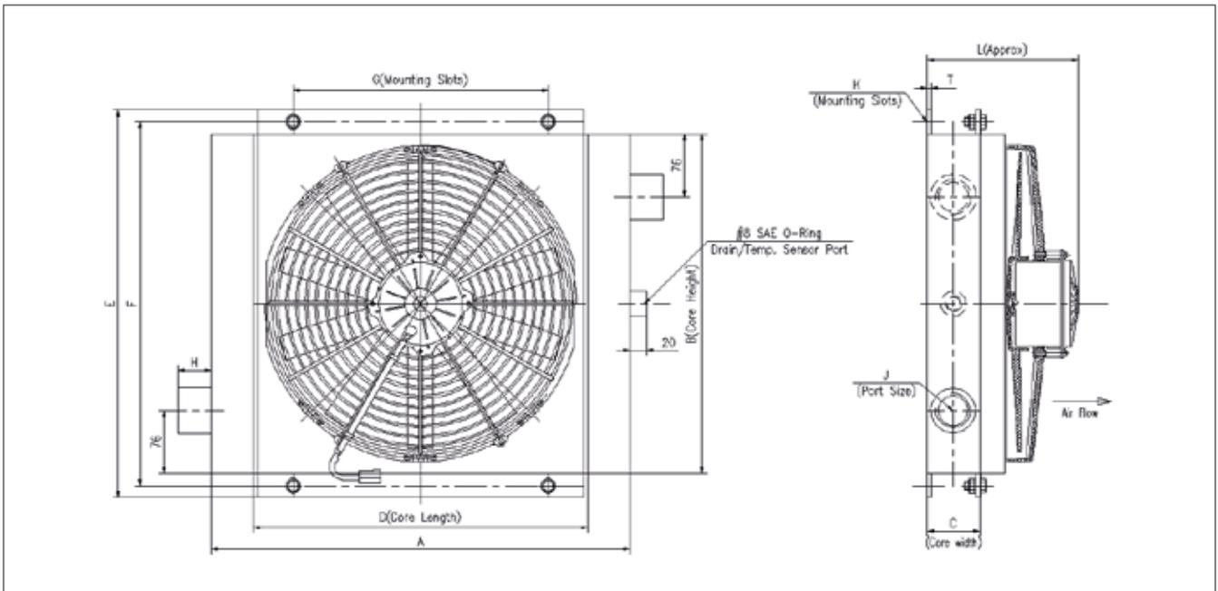
**!** All dimensions are given in mm. Inlet and outlet connections of oil can be reversed.
