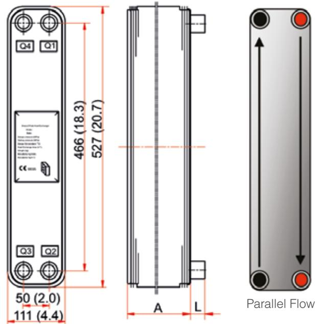
MIT MB-08 can be copper or nickel brazed heat exchanger. Plate material 316L.
