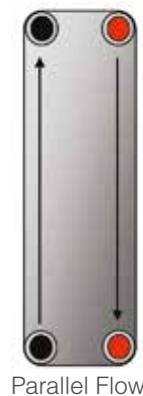
MIT MB-09 can be copper or nickel brazed heat exchanger. Plate material 316L.
