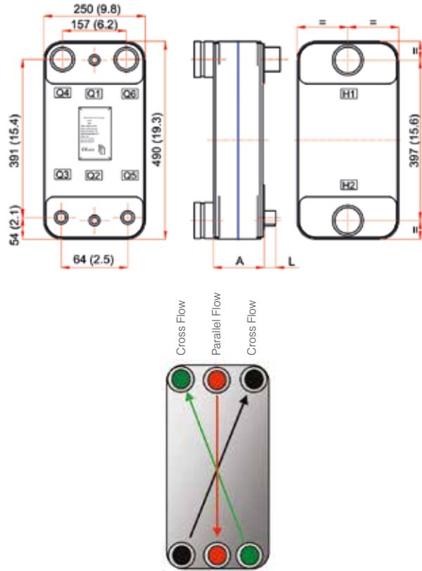
MIT MB-10 can be copper or nickel brazed heat exchanger. Plate material 316L.
