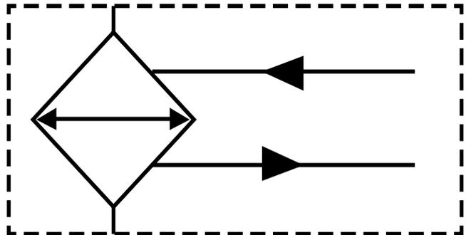
Bypass option of AIB Cooling element for high viscosity applications.
