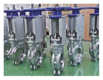
They provide full sealing with their one-piece body and elastromer (EPDM, NBR, NR) seat. They can also be produced with metal seat depending on their fluid properties. They can be flywheel, gear box, chain wheel, pneumatic actuator and electric actuator.
